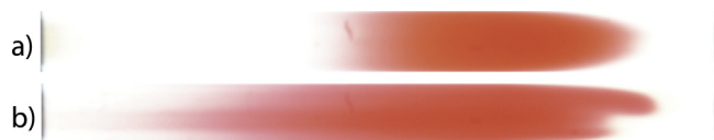
Fig. 7. Photographs illustrating the change in band-shape as a function of the viscosity contrast. In this experiment the refractive index system was matched with the stationary phase, so that the column becomes transparent. In both cases the viscosity of the injection plug was 0.38 cP. The injection volume was 5 \mu L, flow rate 0.5 mL/min. The column internal diameter was 5 mm, and the column length was 54 mm. Flow direction is from left to right. In (a) mobile phase viscosity 0.38 cP, viscosity contrast around 0 and in (b) mobile phase viscosity 1.44 cP, viscosity contrast about 3.8 times.
